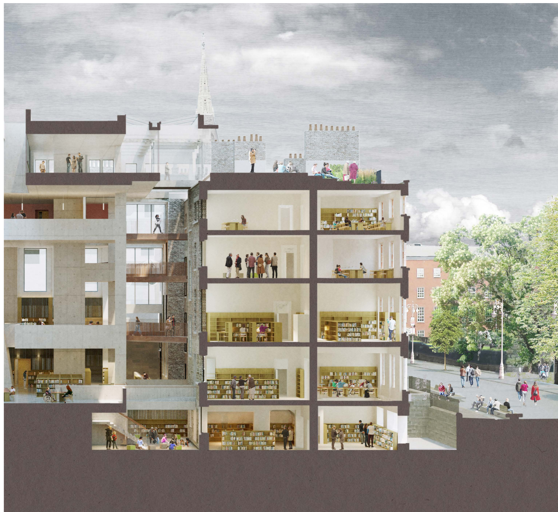
Sectional Perspective View Showing Connection Between New Building & The 18th Century Houses
